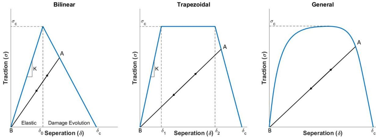
Figure 5: Bilinear, trapezoidal, and general traction-separation relations.
