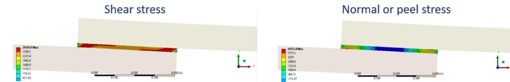
Figure 1: The general process for modeling an overlap shear bond. First the geometry is defined, and material properties are assigned. Then the geometry is broken into elements in a process called meshing. Finally, boundary conditions are applied and the problem is solved.
