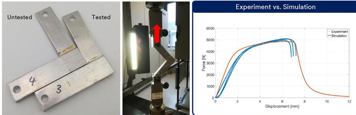
Figure 8: Material model validation using the 90° double lap shear test.
