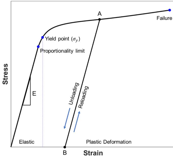
Figure 3: Ductile Structural Adhesives undergo significant plastic deformation prior to failure.
