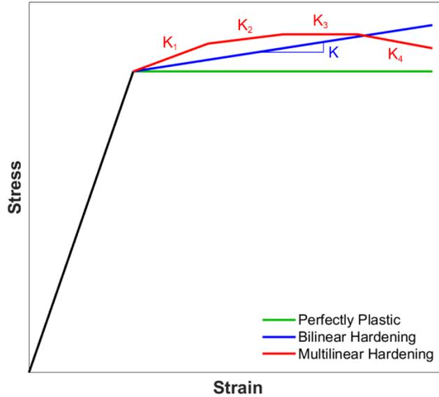
Figure 4: Plastic deformation can be approximated with perfectly plastic, bilinear, and multilinear hardening rules
