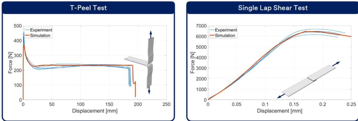
Figure 7: Material model validation using the T-peel and single lap shear tests.
