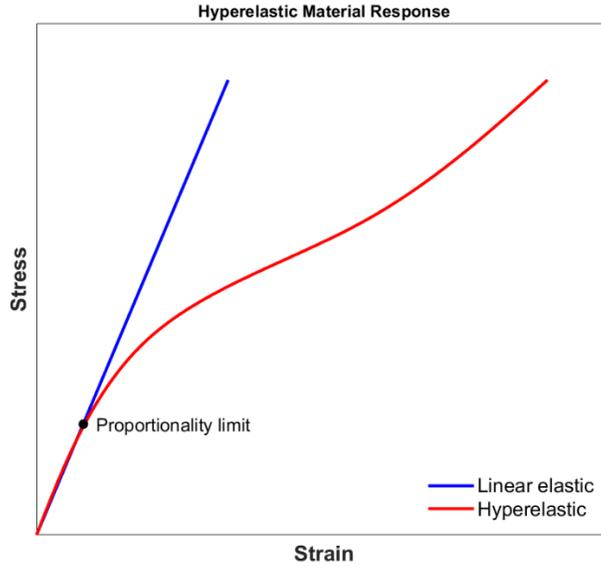
Figure 2: Hyperelastic materials undergo large nonlinear elastic deformations.
