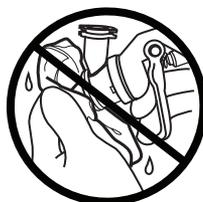
Do not use metal tools to clean the air cap holes as this may scratch them; scratches can distort the spray pattern.
