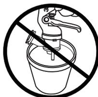
Do not wipe the spray gun with a cloth soaked in solvent; wring out the excess.
