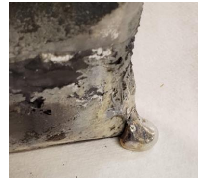
Molten cell containers allow for cell to cell shorting
