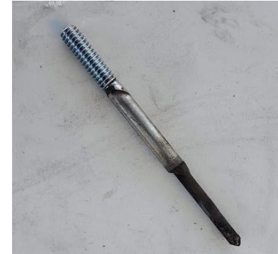
Nail used in thermal runaway testing
