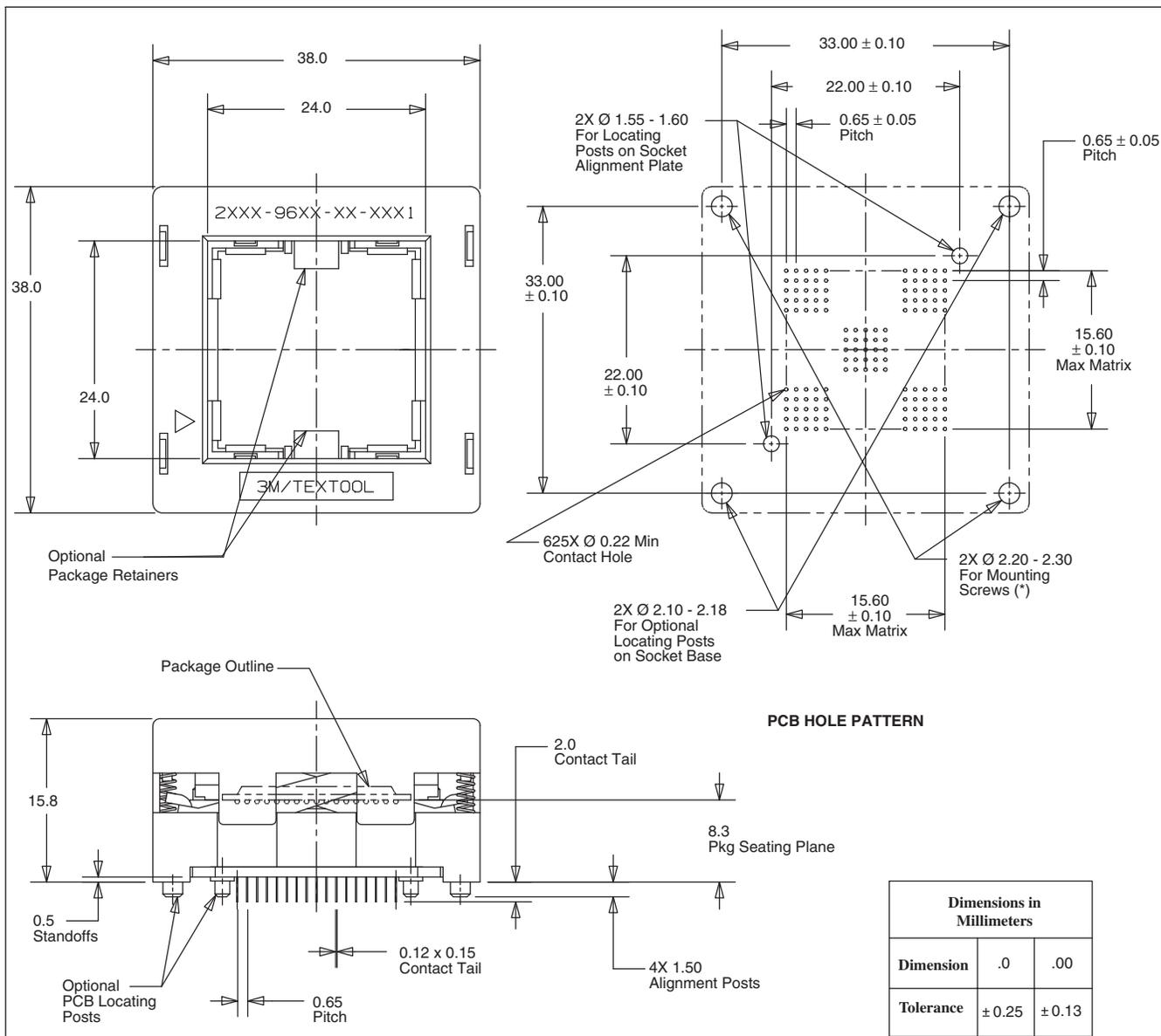
\* For 1.6 mm thick PCB, use self-tapping, STN.STL. screws size M2 x 4.0 mm long.
