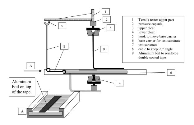
The result is given in a peel force (N) per length (typically 10mm).
