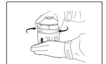
**5** Attach spray gun to filled 3M™ PPS™ Series 2.0 Spray Cup System cup.
