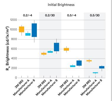
3M™ Diamond Grade™ Conspicuity Markings Series 983 change the least during 2,000 hours of accelerated weathering.\*
