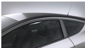
Door Pillars and Window Sashes
