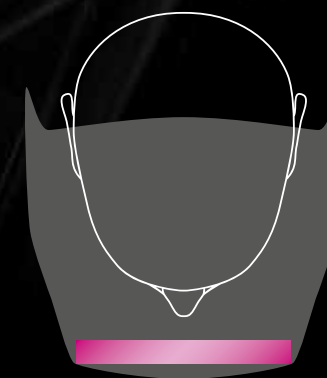
Expanded field of view with a flat ADF requires a wider helmet.
