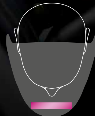
Flat ADF in a slim helmet means the ADF can't be wide.
