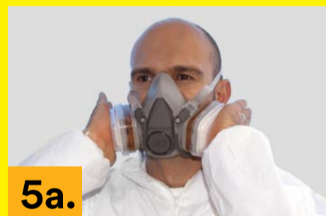
5a. With cartridges: Place the palms of your hands over the cartridges to restrict the air flow. Inhale gently. The facepiece should collapse slightly.
