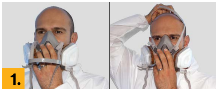
1. Place the respirator over the mouth and nose. Pull the head harness over the crown of the head
