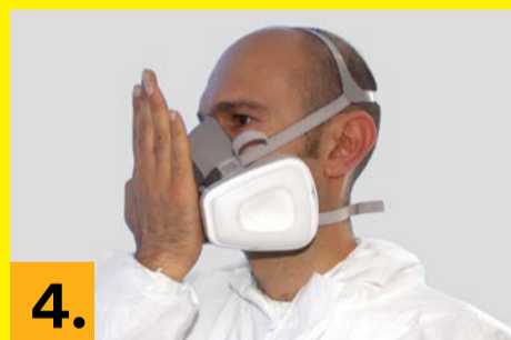
4. Place the palm of your hand over the exhalation valve cover and exhale gently. If the facepiece bulges slightly and no air leaks are detected between the face and the facepiece, a proper seal has been obtained.
