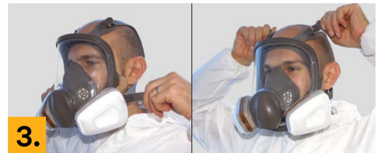
3. Tighten the two bottom straps and then the top straps. Recheck all straps to ensure that they are tight and evenly tensioned so that the head harness is centred on the back of your head.
