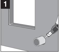
Prep window opening and penetrations. Caulk gaps and ensure all mortar joints are struck flush. Gaps wider than 1.3 cm (0.5 in) must be filled with backer rod and caulk prior to applying 3M<sup>™</sup> Ultra Conformable Flashing Tape 3015UC.
