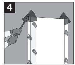
Apply 3M<sup>™</sup> Ultra Conformable Flashing Tape 3015UC in the corners, extending over the vertical sides of window flashing and directly to the wall. Ensure tape is applied with a 5 cm (2 in) minimum overlap in all directions.
