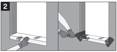
If  $3M^{\mathbb{W}}$  Air and Vapour Barrier 3015 will be used as the sill flashing tape, first cut it the width of the window and apply over the sill extending at least 5 cm (2 in) onto the wall. Then apply  $3M^{\mathbb{W}}$  Ultra Conformable Flashing Tape 3015UC in the corners, extending over the sill tape and up the vertical side of the frame ensuring a minimum 5 cm (2 in) overlap in all directions. Apply pressure with a J-roller.
