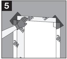
To complete the window detailing, cut a piece of 3M<sup>™</sup> Air and Vapour Barrier 3015 the same width as the window. Overlap a minimum of 5 cm (2 in) onto the wall and over the 3M<sup>™</sup> Ultra Conformable Flashing Tape 3015UC in the upper corners.
