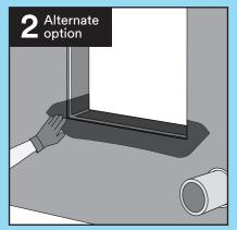
Sill Flashing — 3015UC Only A 22.9 cm (9 in) wide strip of 3M<sup>™</sup> Ultra Conformable Flashing Tape 3015UC can be applied across the entire sill in one continuous piece extending at least 5 cm (2 in) onto the wall and up the vertical sides of the frame.
