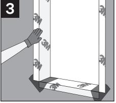
To detail the vertical sides of window, cut  $3M^{**}$  Air and Vapour Barrier 3015 the same length as the height of the frame. Extend onto the wall and overlap the sill flashing a minimum of 5 cm (2 in) to prevent negative laps.
