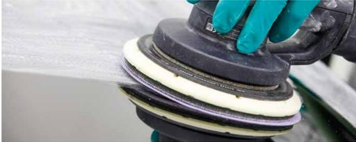
▶ Sand the area with 3M™ Hookit™ Purple Finishing Film Abrasive Disc 260L, grade P1500 - P2000.
