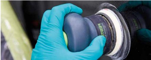
▶ Refine scratches with 3M™ Trizact™ Fine Finishing Disc 443SA, grade 8000, 75mm on orbital sander.
