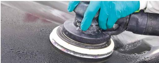
▶ Refine scratches with 3M™ Trizact™ Fine Finishing Disc 443SA, grade 3000, 150 mm on orbital sander.
