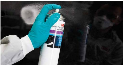
▶ Should sanding scratches from the first polishing step still be visible after controlling the surface, please repeat polishing step!
