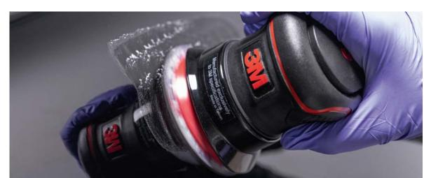
► Scratch refinement with 3M<sup>™</sup> Trizact<sup>™</sup> Fine Finishing Disc 443SA, grade 5000, 75 mm on orbital sander.
