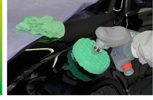
► Add a small amount of 3M<sup>™</sup> Perfect-It<sup>™</sup> Fast Cut Plus Extreme onto the green foam pad on the rotary polisher.
