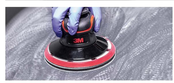
► Sand the area with 3M<sup>™</sup> Hookit<sup>™</sup> Purple Finishing Film Abrasive Disc 260L, grade P1500 - P2000.
