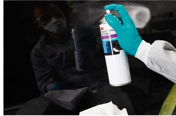
► Should sanding scratches from the first polishing step still be visible after controlling the surface, please repeat polishing step!
