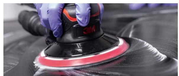
► Sand the area with 3M<sup>™</sup> Trizact<sup>™</sup> Fine Finishing Disc 443SA, grade 3000, 150 mm on orbital sander.
