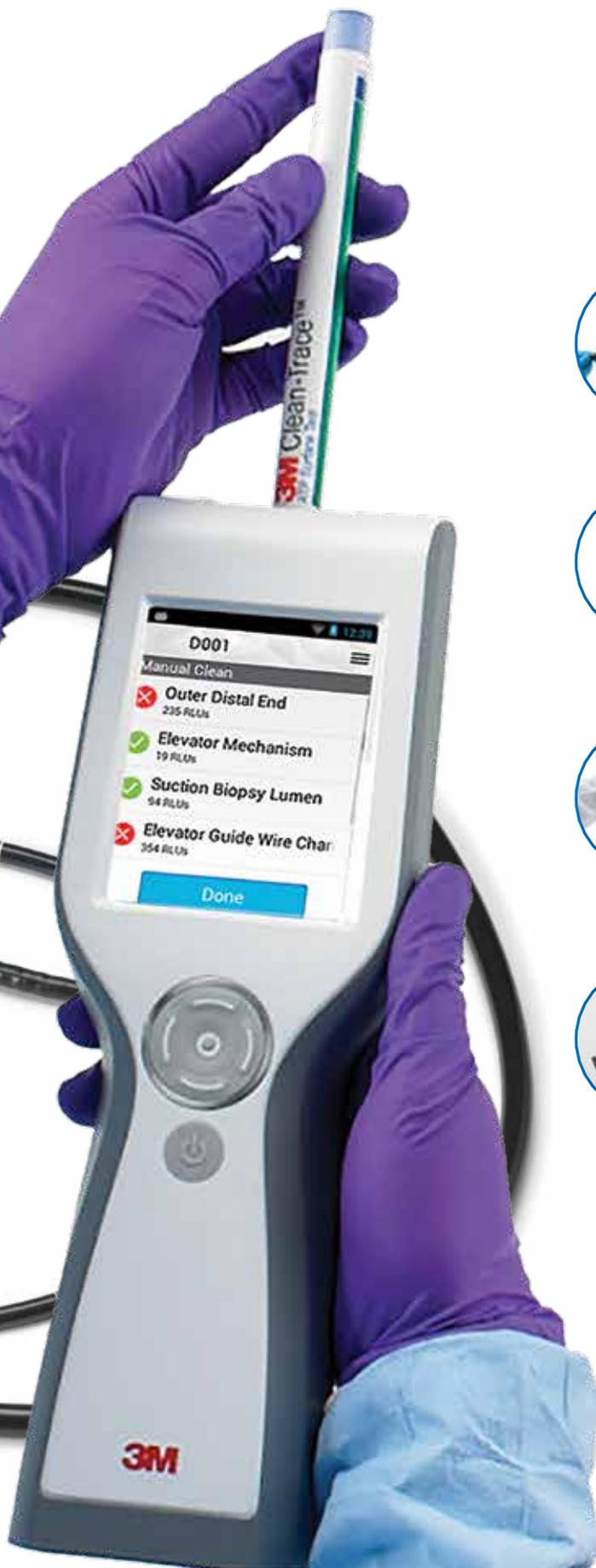
The 3M™ Clean-Trace™ ATP System provides a quality control monitoring tool for difficult to clean medical devices, like flexible endoscopes.
