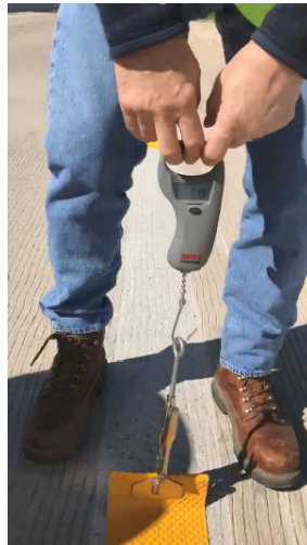
Figure 10. Grip tape firmly with both hands while standing astride the marking.
