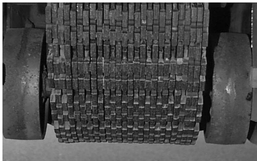
Figure 4. Gang-stacked diamond cutting head.
