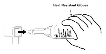
3. Insert assembly into rear of applicator. Fasten end cap securely onto applicator, carefully aligning end cap threads to prevent binding. (If you are completing the setup and installation procedure, wait five (5) minutes to allow nozzle to warm to proper temperature.)
