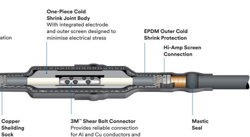
Provides reliable connection for AI and Cu conductors and enables size/type transition without special tools or extra components
