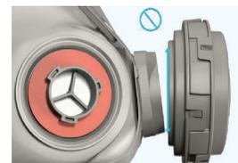
4. If the EVF is not seated evenly on the valve cover, as shown above, in Fig. 4, repeat steps 2 & 3.
