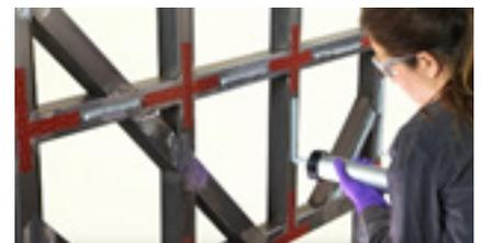
For example, this floor panel assembly was bonded with 3M™ VHB™ Tape 4991 which gives instant adhesion and defines a minimum thickness. 3M™ Hybrid Adhesive Sealant 760 was used for gap-filling where needed.
