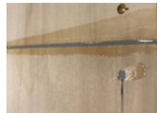
Adhesives can be used to seal the gaps between floor panels. For example, here adhesives from the 3M™ Scotch-Weld™ range are used for bonding (Metal Bonder Acrylic Adhesive DP8407NS and Epoxy Adhesive DP7240) along with 3M™ Hybrid Adhesive Sealant 760.
