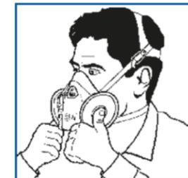
**Fit testing:** The 3M 7500 Half Mask is a tight fitting facepiece and therefore wearers require a fit test as per the COSHH regulations 2002. For qualitative testing – 3M™ FT10 and FT30 Fit Test Kits are available.
