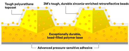
A cross-section of 3M<sup>™</sup> Stamark<sup>™</sup> Pavement Marking Tape Series 380 shows 3M's advanced technologies in every aspect of construction, inside and out.
