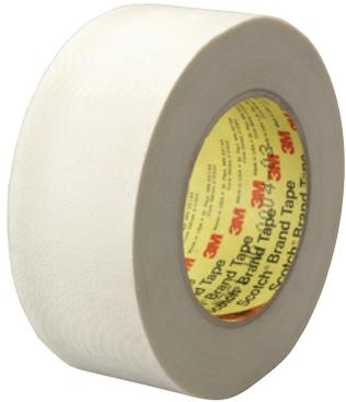
Constructed with a woven fibreglass backing, 3M™ Glass Cloth Tape 361 features a pressure sensitive silicone adhesive for applications requiring high-temperature resistance, high adhesion and clean removal. It is often used for high temperature applications such as sealing ducts and as a back-up strip for submerged arc welding.
