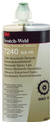
3M™ Scotch-Weld™ 7240 FR B/A epoxy adhesive is a toughened, two-part epoxy adhesive with a 2:1 mix ratio, 45 minutes work life and handling strength in approximately 6 hours. This product is very durable and commonly used in applications in the transportation industry. With high peel and shear strength 3M™ Scotch-Weld™ Epoxy Adhesive 7240 FR maintains lasting bonds in tough environmental conditions. It works well on metals and many composites.
