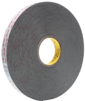
A thick, grey, double-coated acrylic foam tape with paper liner. The multi-purpose acrylic adhesive on both sides bonds to a broad range of high and medium surface energy substrates including metals, glass and a wide variety of paints and plastics. The conformable foam provides good contact between substrates even when they are slightly mismatched. Fast and easy-to-use permanent bonding method provides high strength and long-term durability
