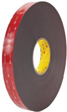
A modified acrylic adhesive on both sides bonds to a broad range of high, medium and medium/low surface energy substrates including metals, glass and a wide variety of plastics and paints, including many powder coated paints. The very conformable foam provides good contact between substrates even when they are slightly mismatched.
