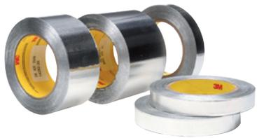
A foil tape for numerous applications across a broad range of industries. Comprised of a dead soft aluminium foil backing and coated with a highly engineered pressure sensitive acrylic adhesive, it is ideal for heat shielding, heat reflecting, chemical masking, light enhancement, chemical milling, seaming, sealing and de-paint operations
