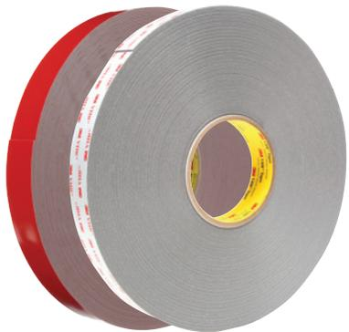
The multi-purpose acrylic adhesive on both sides bonds to a broad range of high and medium surface energy substrates including metals, glass and a wide variety of paints and plastics as well as plasticised vinyl. The conformable foam provides good contact between substrates even when they are slightly mismatched.
