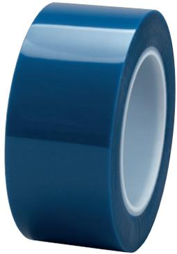
A general purpose polyester tape ideal for masking in high temperature applications. Coated with a silicone adhesive, this tape functions well in masking for powder coating and anodising to provide sharp paint lines. It removes cleanly and in one-piece from most surfaces, avoiding slivering and breaking.
