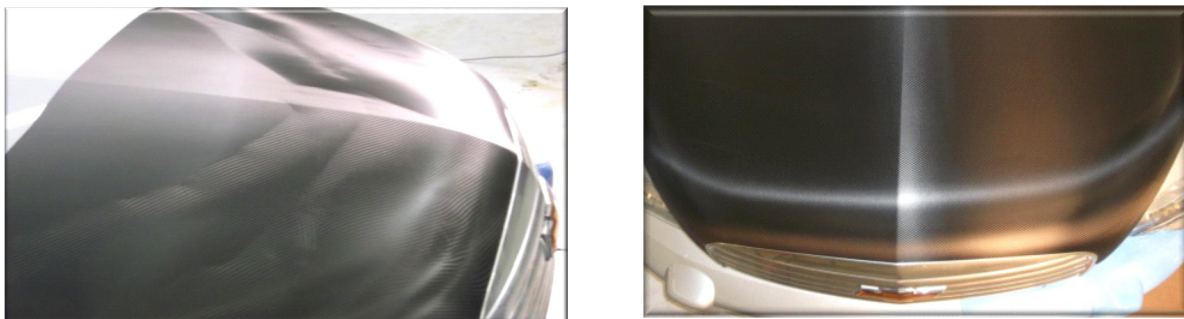
Figure 2. Damaged Film vs. Undamaged Film Post-Installation
