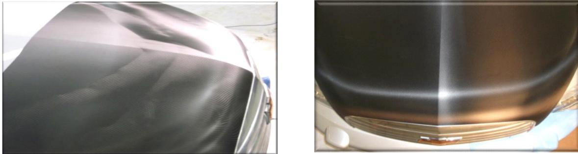
**Figure 2.** Damaged Film vs. Undamaged Film Post-Installation
