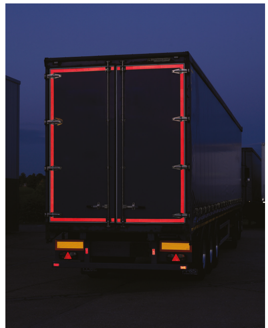
Conspicuity tapes applied as a complete contour line marking (box) on the rear of a trailer.
