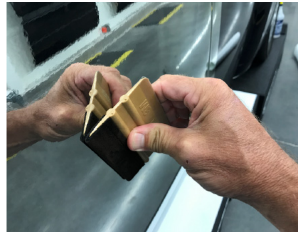
Figure 2. Use dampened, soft-sided squeegee for application. Always ensure soft side is saturated with a slip solution.
