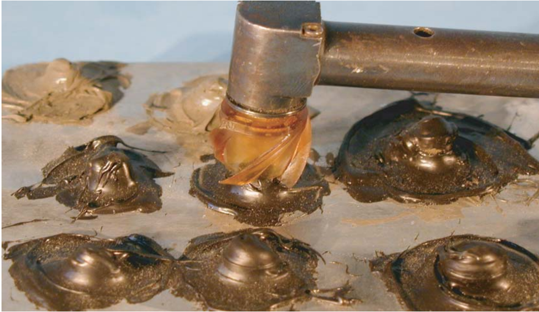
Removal of sealant from fasteners
