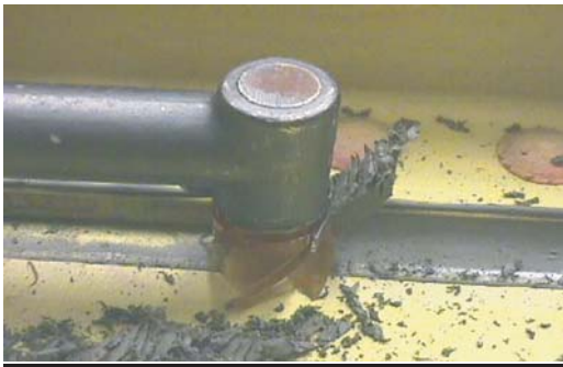
Cleaning fillet with the bottom of the SR Cutter
