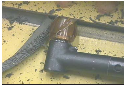
Cleaning fillet with the side of the SR Cutter
