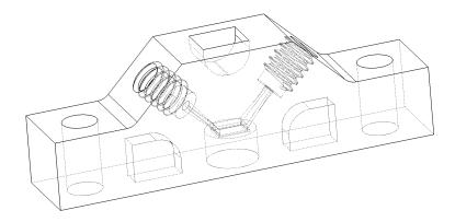
The reaction chamber had to be custom-designed and built to accommodate the electronic components used in their research that tend to be inflexible and come in a large variety of unique shapes. With the flexibility of additive manufacturing, Polymer Forge can prototype multiple chamber designs with complex internal features to test varying electronic components quickly, eliminating complexity constraints of traditional manufacturing.
