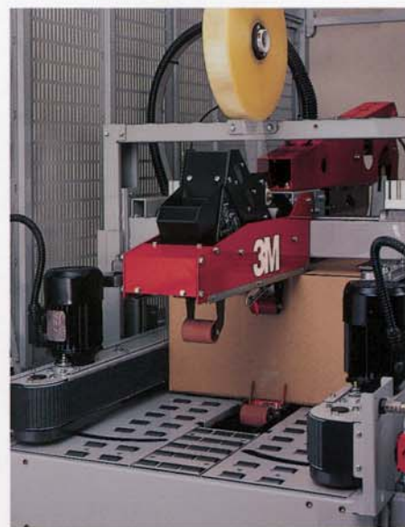
Self-centering laced side belts grip cases for positive drive and consistent tape application.
