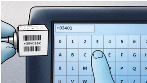
5. The scaling factor is shown on each block and must be entered into the system prior to milling.
