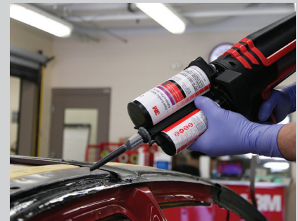
May be used for bonding door skins, quarter panels, roof skins, box sides, van/utility vehicle sides and sills when recommended by OEMs.
