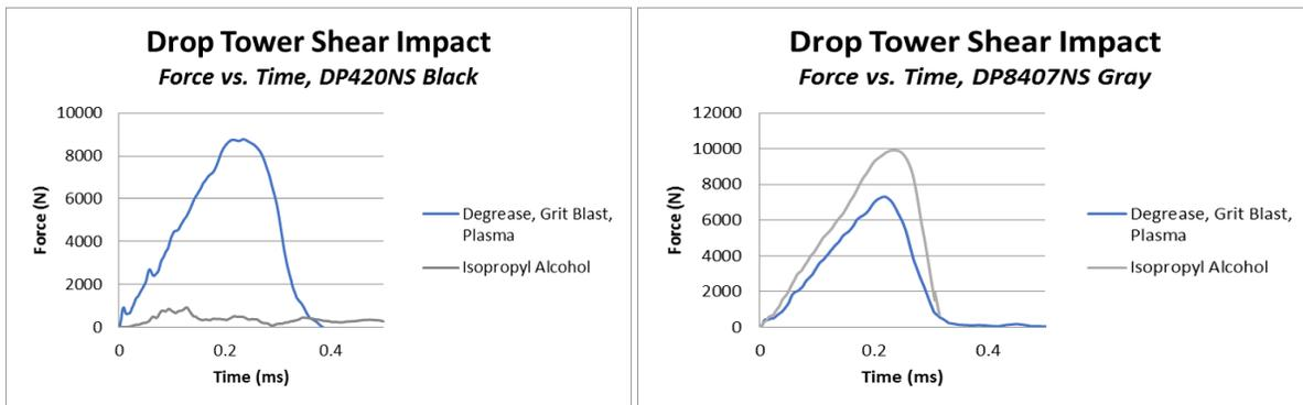
Figure 8-9: Force vs. Time curves for DP420NS Black and DP8407NS Gray comparing different surface preparations bonding 6061 aluminum. Average curves reported.
