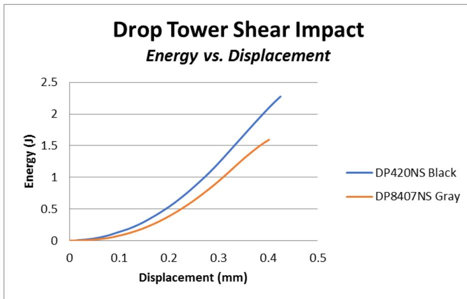
Figure 7: Energy vs. Displacement curves for DP420NS Black and DP8407NS Green. Samples were solvent degreased, grit blasted, and plasma treated prior to bonding. Average curves reported.
