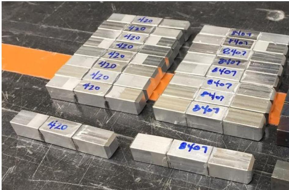
*Figure 3: Bonded impact specimen using DP420NS Black and DP8407NS Gray.*
