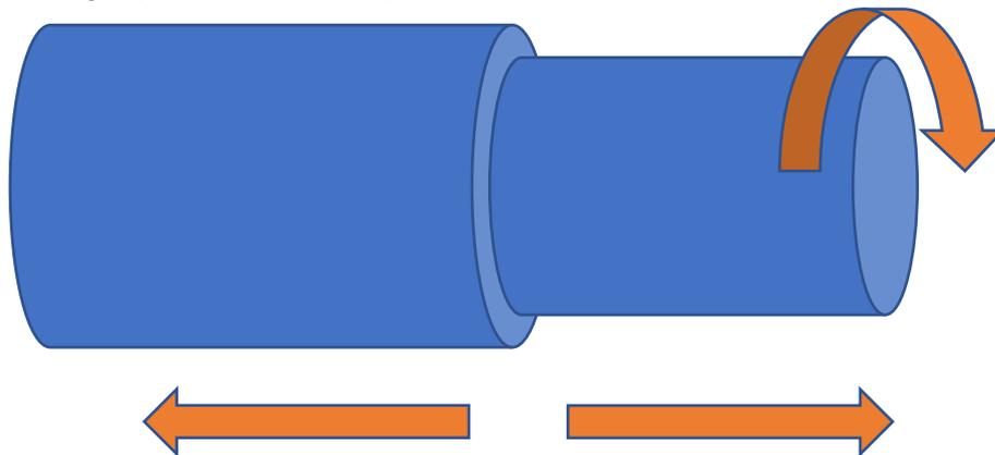
*Figure 1: Representation of a bonded tube-in-tube assembly that maintains shear loading of the adhesive bond line.*
