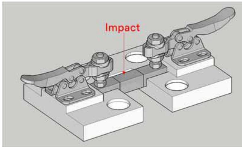
Figure 2: Fixture holder and adhesive geometry used during a shear impact event.
