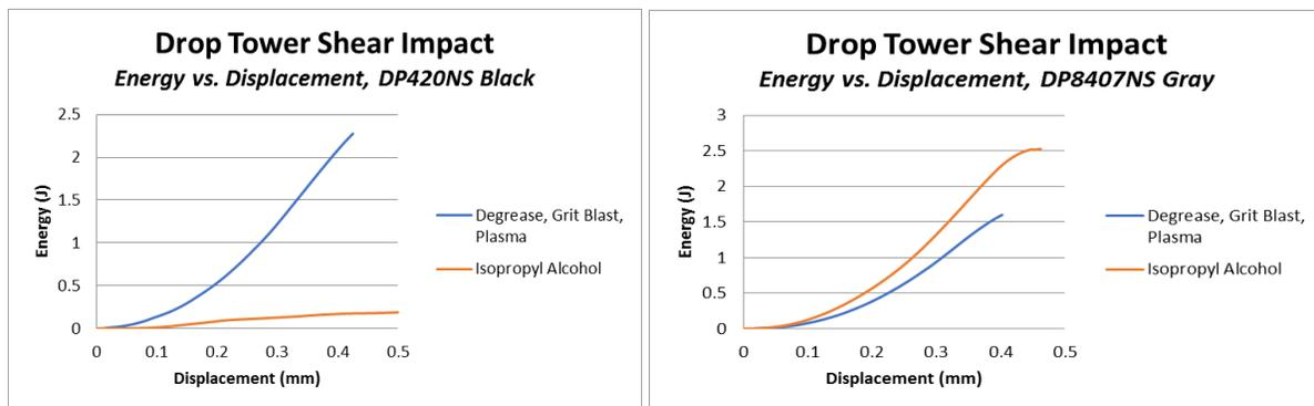
Figure 10-11: Energy vs. Displacement curves for DP420NS Black and DP8407NS Green comparing different surface preparations bonding 6061 aluminum. Average curves reported.
