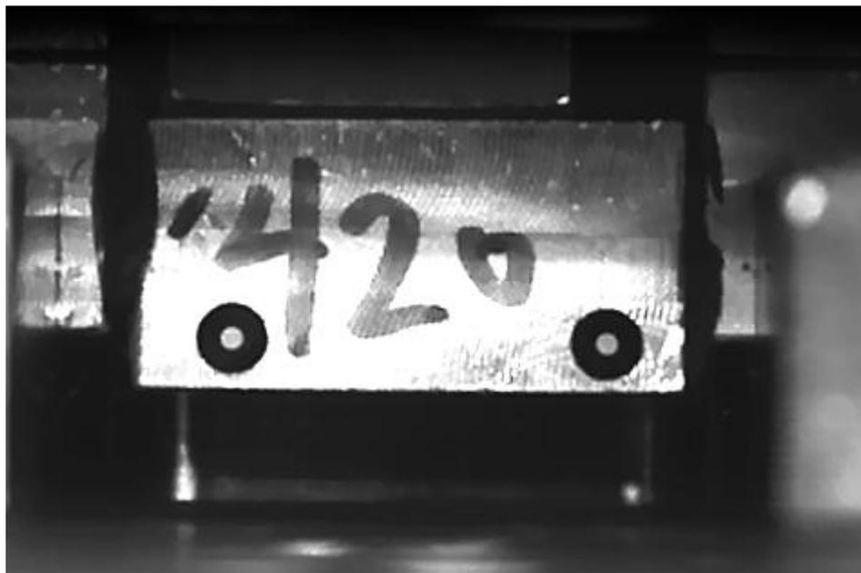
*Figure 5: Screen capture of the DP420NS Black failing under shear impact.*
