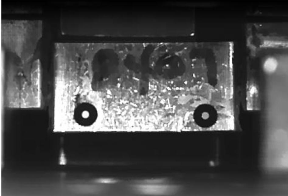
*Figure 4: Screen capture of the DP8407NS Green failing under shear impact.*
