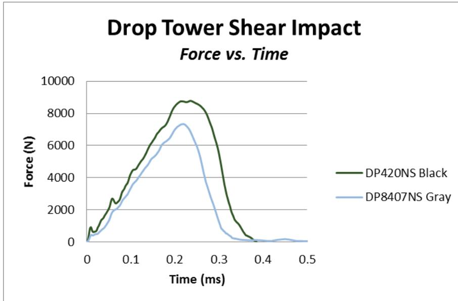
Figure 6: Force vs. Time curves for DP420NS Black and DP8407NS Green. Samples were solvent degreased, grit blasted, and plasma treated prior to bonding. Average curves reported.
