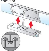
Easily overcome variability in panel or trim size for ceilings and side panels; no screw alignment needed. Removable for service or refurbishment.
