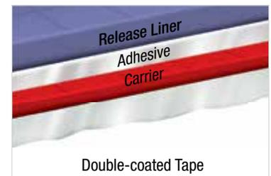
A spacer tape is a double-coated tape manufactured for microfluidic test strips. This tape has a precise overall thickness that provides gapping, channel height thickness, and structure to the test strip.
