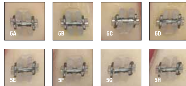
Figure 5A-H: Bonded samples exposed to curry broth for 240 minutes at 40°C
