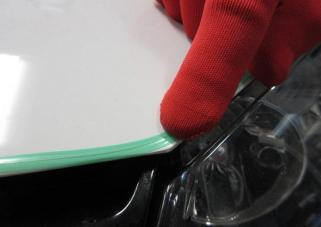
The use of special application tools helps to remove air underneath the tape.
