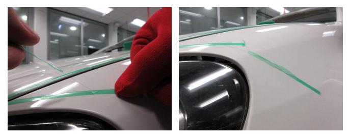
For corners it is recommended to apply several stripes of 3M<sup>™</sup> Knifeless Tape and to mark the order of application.
