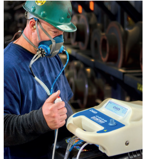
Figure 3 - Controlled Negative Pressure - OHD® Quantifit® CNP using the REDON method being used to conduct a Quantitative Fit Test (QNFT) upon a subject wearing a filtering facepiece respirator. Image: courtesy of OHD®
