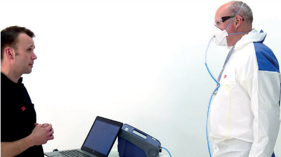
Figure 2 - Ambient Particle Counting - TSI® PortaCount® Respirator Fit Tester Model 8038 being used to conduct a Quantitative Fit Test (QNFT) upon a subject wearing a filtering facepiece respirator
