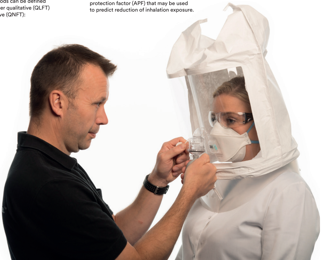
Figure 1 - 3M™ Qualitative Fit Test Apparatus Kit and Bitrex® Fit Test kit being used to conduct a Qualitative Fit Test (QLFT) upon a subject wearing a filtering facepiece respirator
