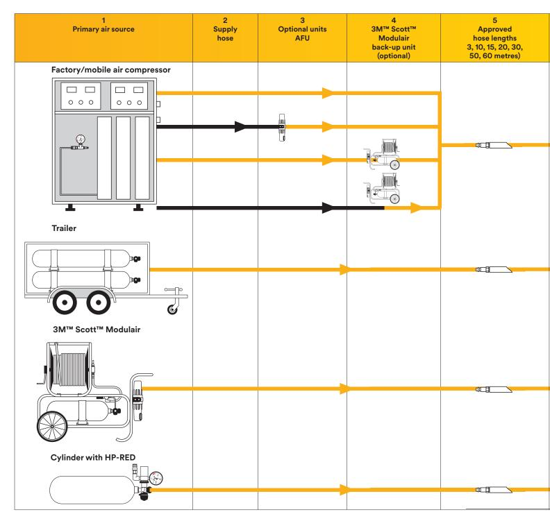
These examples are designed to give an indication of how an airline system can be built up. Please note that many other confgurations can be specified. The line drawings above are only representations of 3M<sup>™</sup> Scott<sup>™</sup> airline equipment and should not be considered exact specification. Maximum length of hose to the user after the 3M<sup>™</sup> Scott<sup>™</sup> Modulair should be no more than 105 metres. Please see Modulair user manual for approved configurations.
