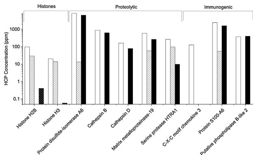
**Fig. 4.** concentration of specific problematic HCPs, in ppm, identified following depth filtration (white bars) and in the subsequent Protein A eluate (light hash bars) compared to FT-AEX clarified material (black bars) and subsequent Protein A eluates obtained with FT-AEX clarified material (dark hashed bars).
