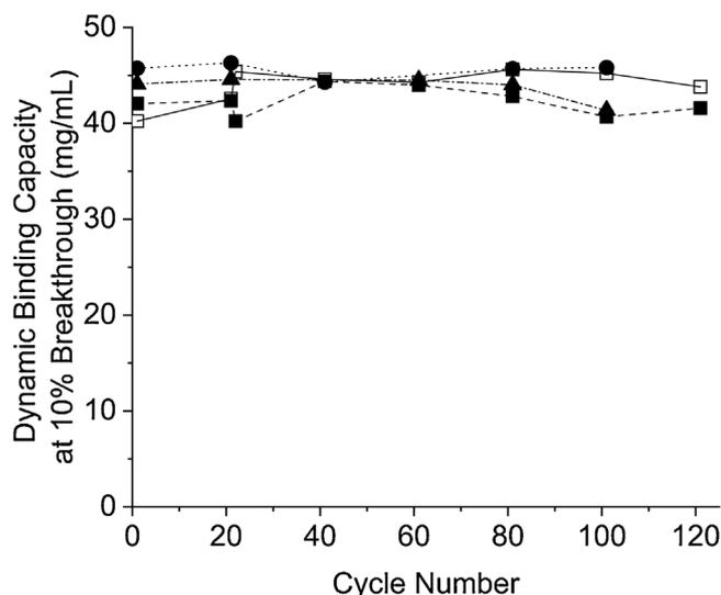
**Fig. 1.** Dynamic Binding Capacity (DBC) at 10% breakthrough for Protein A cycling studies with FT-AEX clarified feed material with no sanitisation (white squares), depth filter clarified material with no sanitisation (black squares), depth filter clarified material with mild sanitisation (black circles) and depth filter clarified material with harsh sanitisation (black triangles).
