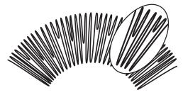
3M<sup>™</sup> High Flow HFR Advanced Pleat Technology utilizes a special configuration to increase the accessible surface area for greater filter media utilization.
