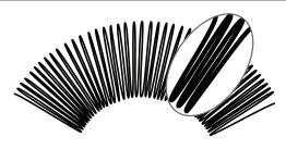
Conventional pleat designs, with full-depth densely packed pleats, fill the upstream pleat surface with contaminant that quickly constrict flow at the pleat's inside diameter.
