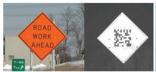
Infrared 2D codes imbedded within a roadway sign that can be read by both the human eye and machine vision
