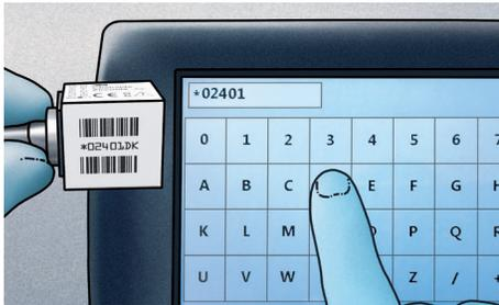
5. The scaling factor is shown on each block and must be entered into the system prior to milling.
