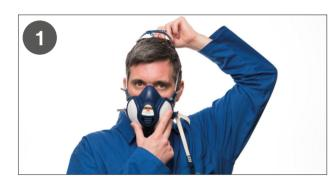
Step 1: Assemble/adjust head cradle by feeding the perforated strip through the buckle and pressing down on the stud at the required length. Repeat for second strip. Place the respirator over the face, fitting it comfortably on bridge of the nose, then pull the head harness over the crown of the head.
