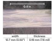
Width and thickness are nominal and not for specification purposes. Thickness was measured under 0.6 psi with a pressure foot gauge.
