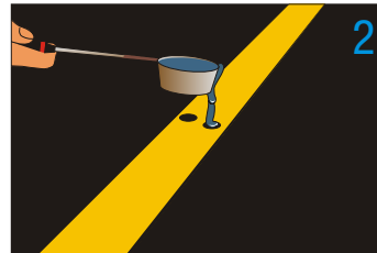
The holes are filled with bitumen
