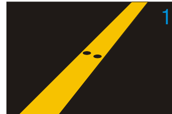
The holes are dug on the bitumen surface
