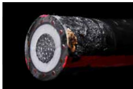
Cable protected with Scotch® Fire Retardant Electric Arc Proofing Tape 77 after test
