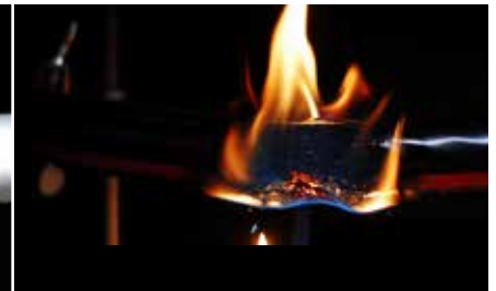
Unprotected cable during test
