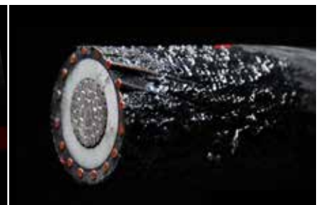
Unprotected cable after test
