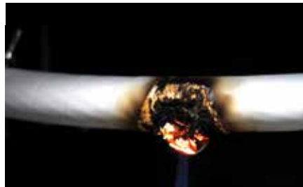
Cable protected with Scotch® Fire Retardant Electric Arc Proofing Tape 77 during test
