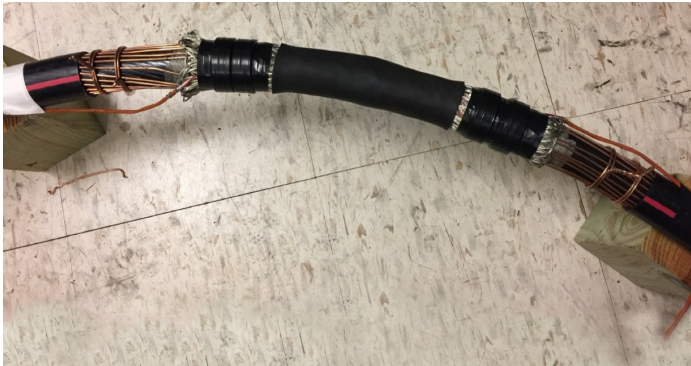
Figure 2: Assembly shielding sock with constant force springs, covered with vinyl electrical tape*
