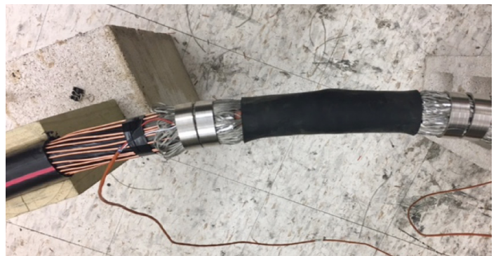
Figure 3: Assembly shielding sock with constant force springs, not covered with vinyl electrical tape*
