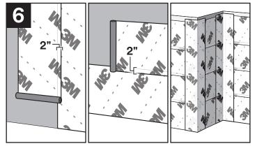
Continue applying  $3M^{\sim}$  Air and Vapor Barrier 3015NP until the entire surface is covered, ensuring a minimum of a 2" overlap. Apply in a shingle fashion starting at the bottom of the wall to prevent negative laps.  $3M^{\sim}$  Air and Vapor Barrier 3015NP can be applied vertically or horizontally as long as there is a minimum 2" overlap. Inside and outside corners require a minimum 2" wide double layer on each wall.
