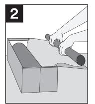
The 3M<sup>™</sup> Air and Vapor Barrier 3015NP box can be used as a dispensing unit. Cut the material to the desired length. There are 6" tick marks that can be used for measuring.
