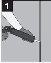
Prepare the wall. Any gaps greater than 1/2" requires backer rod and caulk. Gaps from 1/4"-1/2" require caulk. Concrete walls should have any void areas filled and any fins, mortar joints or screws should be flush with the wall.
