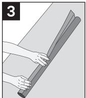
An effective application technique for 3M<sup>™</sup> Air and Vapor Barrier 3015NP is to create a starter strip. To do this, crease the release liner approx 1" and peel back to expose the adhesive on the air barrier.
