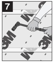
All surface area covered with 3M<sup>™</sup> Air and Vapor Barrier 3015NP requires applying pressure with a squeegee or rolling with a J-roller to ensure a tight bond.
