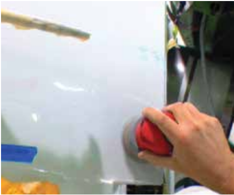
For defects outside the limit, repair by area per Process Step 1, sanding, and Process Step 2 for buffing.
